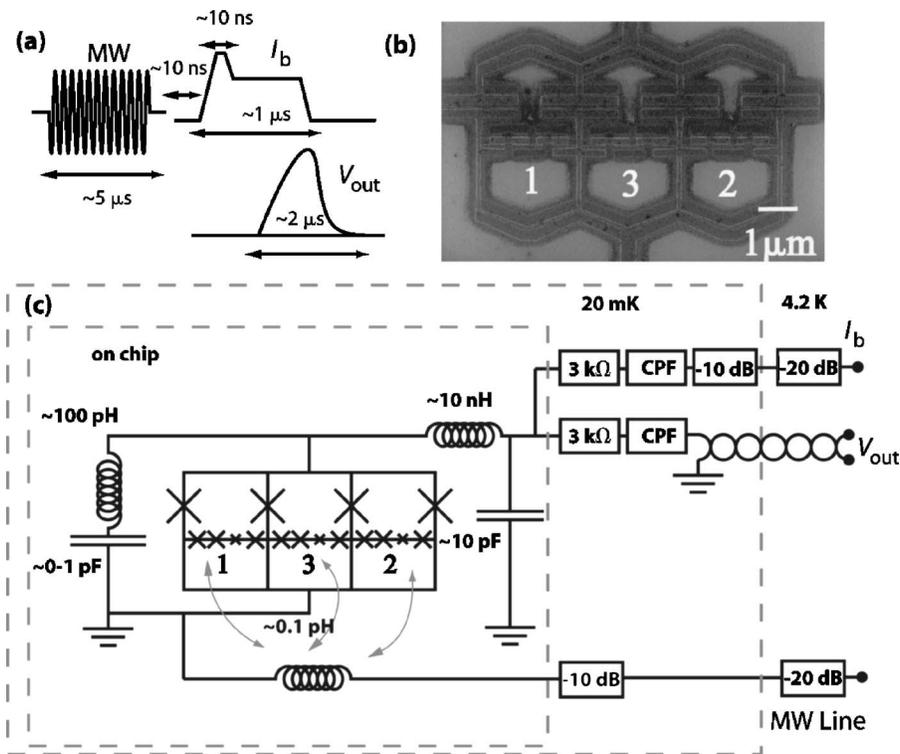
FIG. 1. (a) Timing diagram and the principle of the measurement. (b) Scanning electron microscope (SEM) image of the sample. (c) Detailed wiring. CPF stands for copper powder filter.
